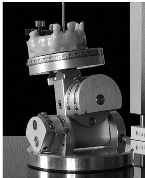
**Fig. 4.** Parallelometer able to transfer the implant position from the virtual project to the master model
