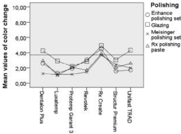
**Fig. 3.** Graphical representation of mean (ΔE) colour changes after repolishing procedures of provisional materials soaked in distilled water (control) for all polishing groups
