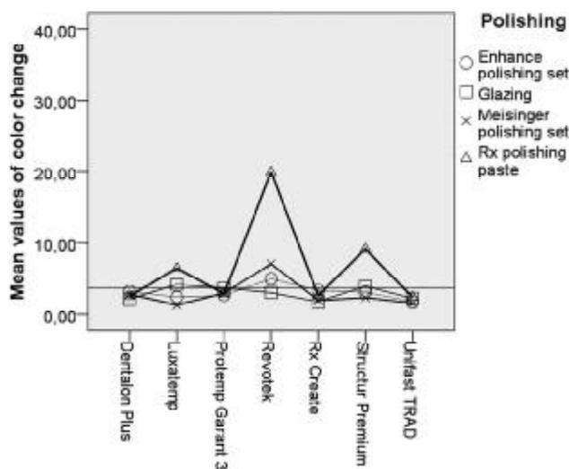
**Fig. 5.** Graphical representation of mean ( $\Delta E$ ) colour changes after repolishing procedures of provisional materials soaked in coffee with sugar for all polishing groups
