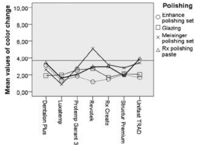
**Fig. 4.** Graphical representation of mean (ΔE) colour changes after repolishing procedures of provisional materials soaked in mix of sunset yellow and quinoline yellow 3% solution for all polishing groups
