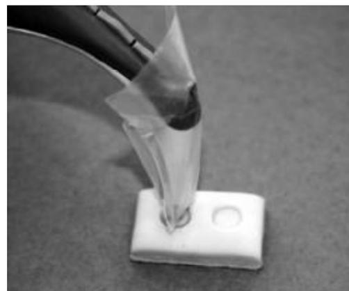
**Fig. 2.** Spectrophotometer tip placed against a specimen in a custom silicone holder
