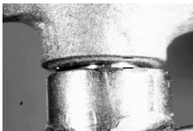
Fig. 2. Marginal discrepancy between the prosthetic component and the implant
